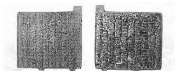
OVERCHARGED NEGATIVE & POSITIVE PLATES
