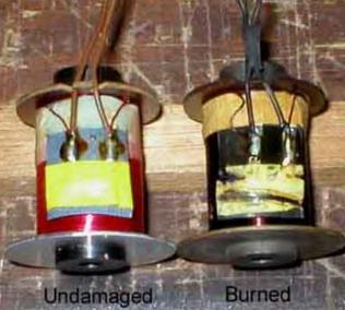
The above description is for a points style fuel pump. The results are even more severe if you have an all electronic pump. I have been told by one of the technicians at Burlen Fuel Systems (makers of all things SU) that when the swamping resistor in the all electronic pumps burns out, the pump won't function at all. Further, if the power is left on long enough while an all electronic pump is stalled in a current on condition, damage will be done to the circuit board.
